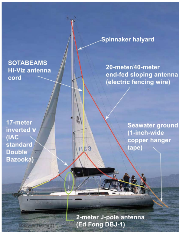
Auriah 's antenna setup. [William Meng, K9TTL, photo]
