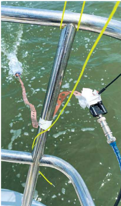
The end of the 20 – 40-meter wire antenna was attached to the aft railing of Auriah with a copper hanging tape counterpoise weighed down by a full water bottle. [Kent Carter, AJ6NI, photo]
